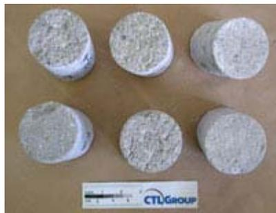
To determine the SRIs of two RCC parking area pavements in Tennessee, three core specimens were obtained from each pavement. At the time of sampling, Pavement 1 and Pavement 2 were about 2 and 10 years old, respectively. Both RCC mixes contained #57 stone, manufactured limestone sand, 400 lbs/yd<sup>3</sup> portland cement, and about 125 lbs/yd<sup>3</sup> Class F fly ash. The cores surfaces were tested in accordance with ASTM C1549-04, *Standard*
